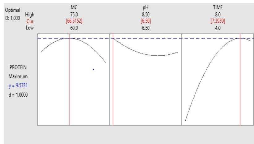
**Figure 4.** Optimum conditions for moisture content, pH and incubation time on Single Cell Protein.
