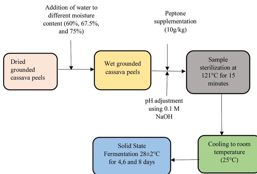
**Figure 2.** Flowchart for fermentation process.
