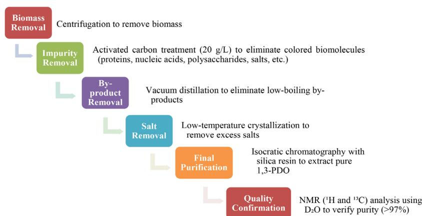
**Figure 4.** 1,3-propanediol recovery process flowchart.
