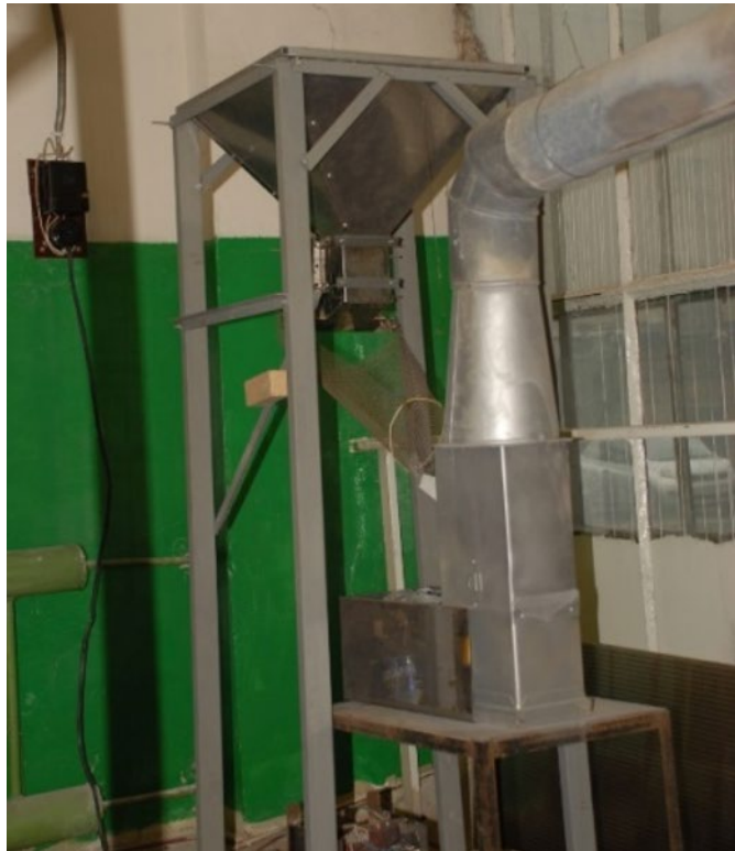
Figure 2. External view of the experimental setup for testing pellet burner with tubular gas heater.
