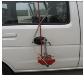
**Figure 11.** Car speed meter.
