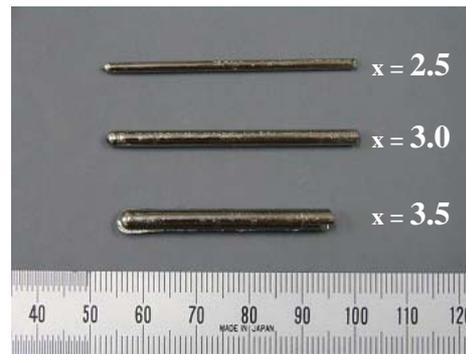
Fig. 3 Photo of as-cast  $(\text{Fe}_{0.5}\text{Co}_{0.5})_{71-x}\text{Gd}_x\text{Nb}_4\text{B}_{25}$  ( $x = 2.5 - 4.5$ ) alloy rods with diameters of 2 to 5 mm.
