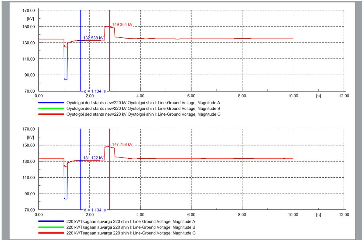
Figure 8. Voltage at the 220 kV side of the Oyu Tolgoi and Tsagaan Suvarga substations during TPAR.
