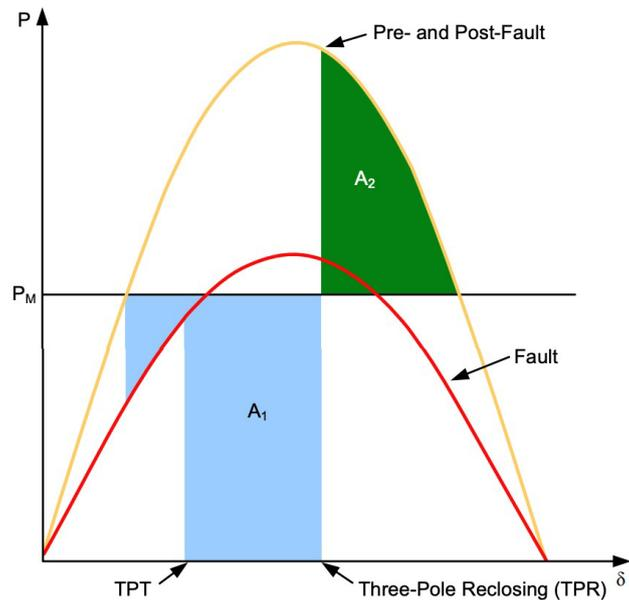
**Figure 2.** Equal area criterion for three-phase disconnection [5].
