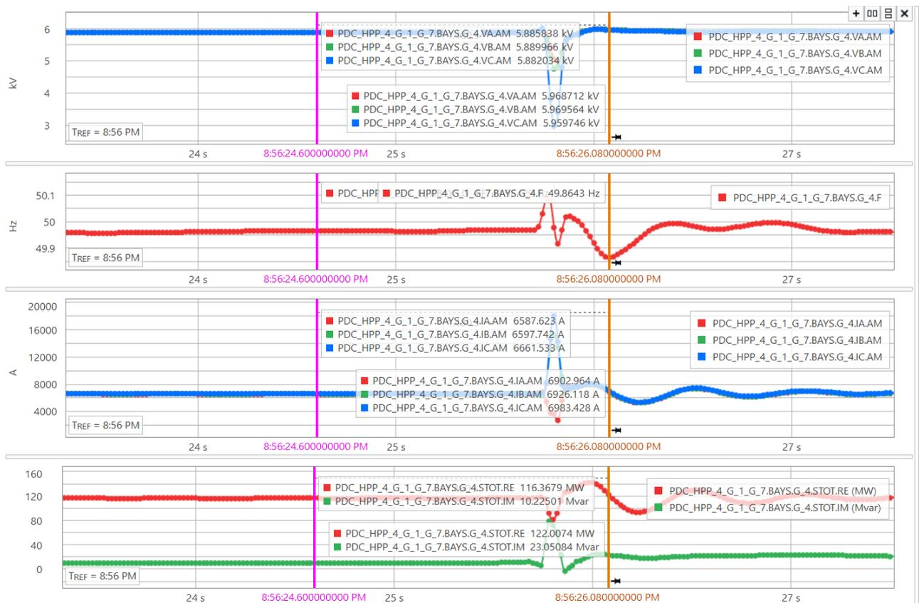
**Figure 11.** Voltage and frequency fluctuations of CHP-4 TG-4 observed on WAMS during single-pole reclosing (TAPV) on L-213 at 08:56:26 on April 20, 2024.
