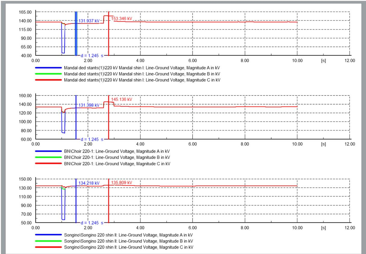
Figure 6. Voltage at the 220 kV side of the Songino, Mandal, Choir substation during TPAR.
