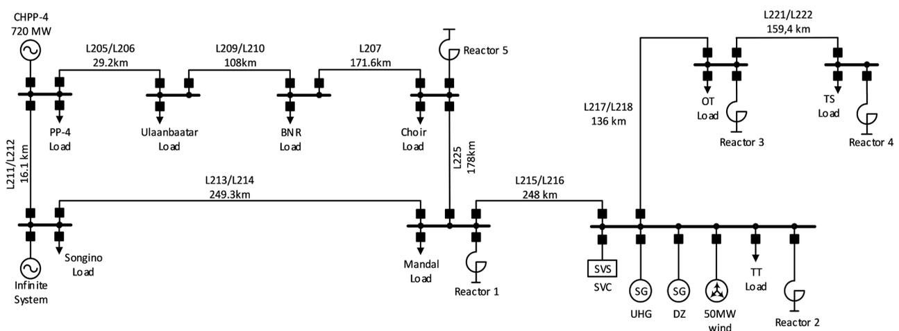
**Figure 1.** General scheme of the network modeled and studied.
