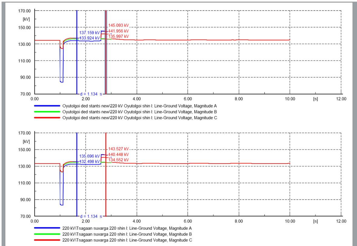
Figure 9. Voltage at the 220 kV side of the Oyu Tolgoi and Tsagaan Suvarga substations during SPAR.
