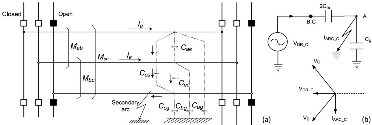
**Figure 10.** Secondary arc ignition and current-voltage vector diagram.
