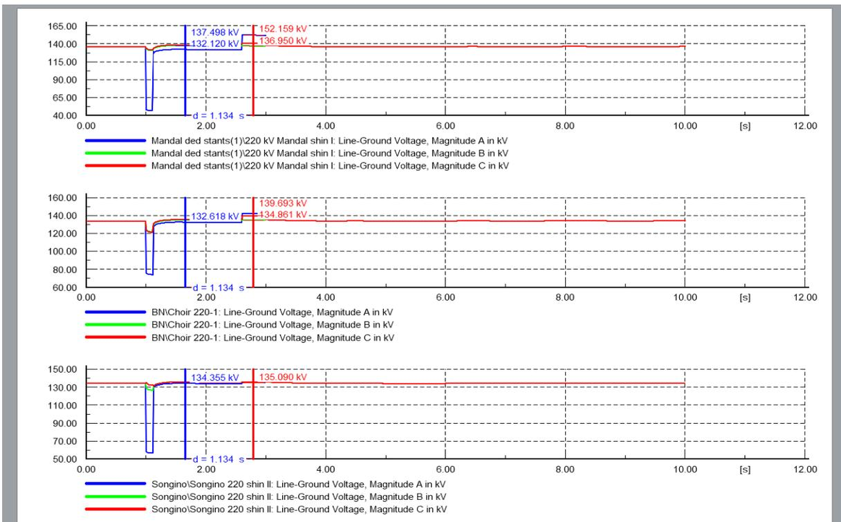
Figure 7. Voltage at the 220 kV side of the Songino, Mandal, Choir substation during SPAR.
