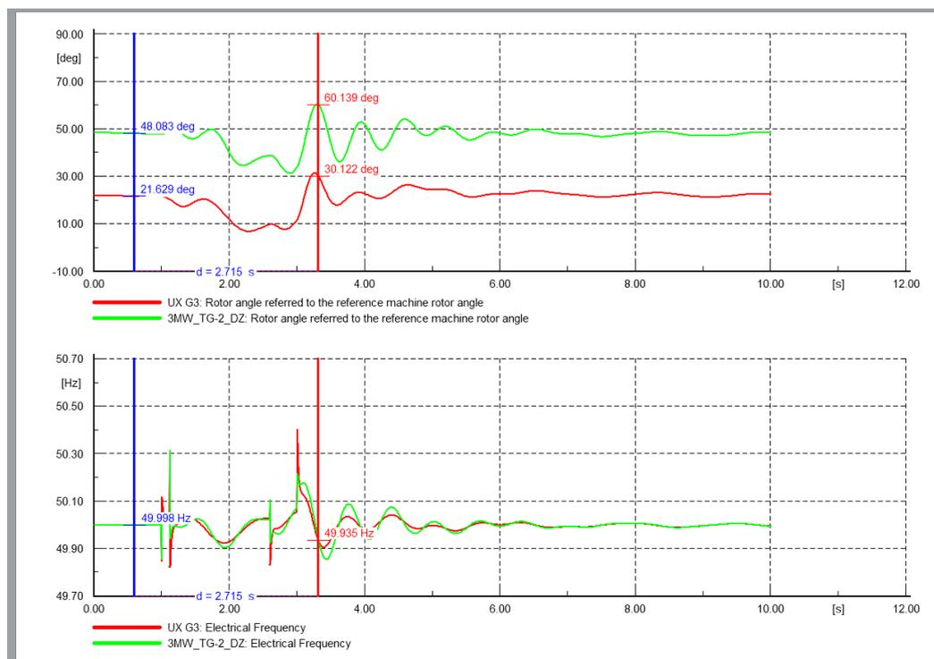
**Figure 4.** Simulation during three phase reclosing: Frequency and rotor angle stability, as well as frequency fluctuations, of Uhaa Khudag TG-3 and Dalanzadgad TG-2.
