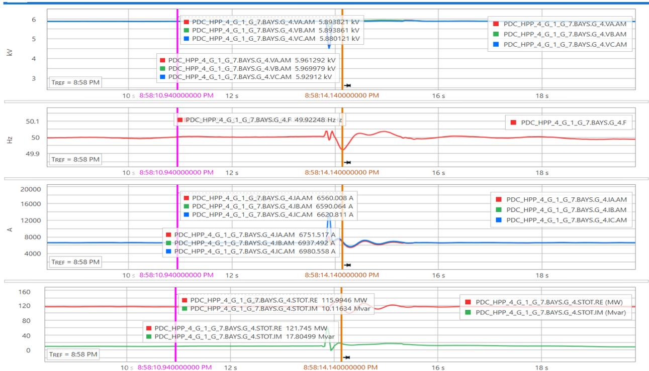
**Figure 12.** Voltage and frequency fluctuations of CHP-4 TG-4 observed on WAMS during auto reclosing (OAPV) on L-213 at 08:58:13 on April 20, 2024.
