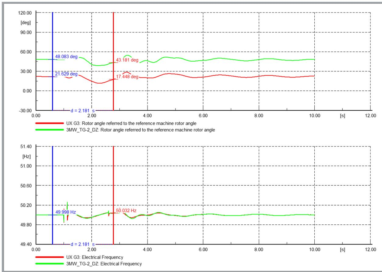
**Figure 5.** Simulation during single-phase automatic reclosing: Frequency and rotor angle stability, as well as frequency fluctuations, of Uhaa Khudag TG-3 and Dalanzadgad TG-2.
