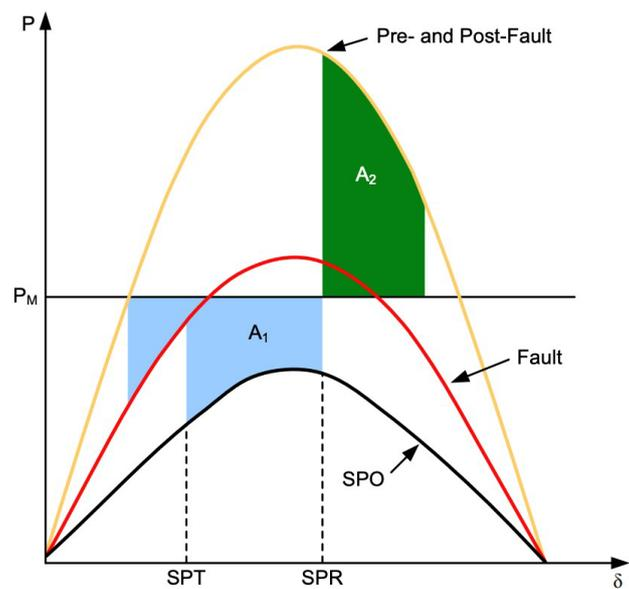
**Figure 3.** Equal area criterion for single-phase disconnection [5].
