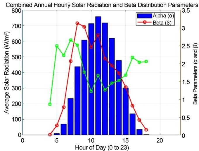
**Figure 6.** Annual hourly solar radiation and beta distribution parameters.
