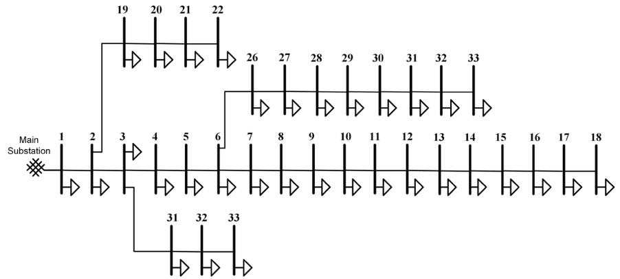
**Figure 5.** Schematic representation of the 33-bus radial test system.
