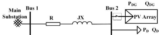
**Figure 1.** Single line diagram of the 2-bus system.
