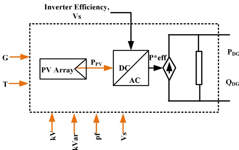
**Figure 2.** General diagram for PV model for Co-simulation.
