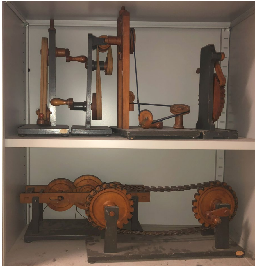
Figure 13. Models from the collection of Bologna University referring to belt and chain transmissions for different axis configurations according to the examples in (Masi, 1897).
