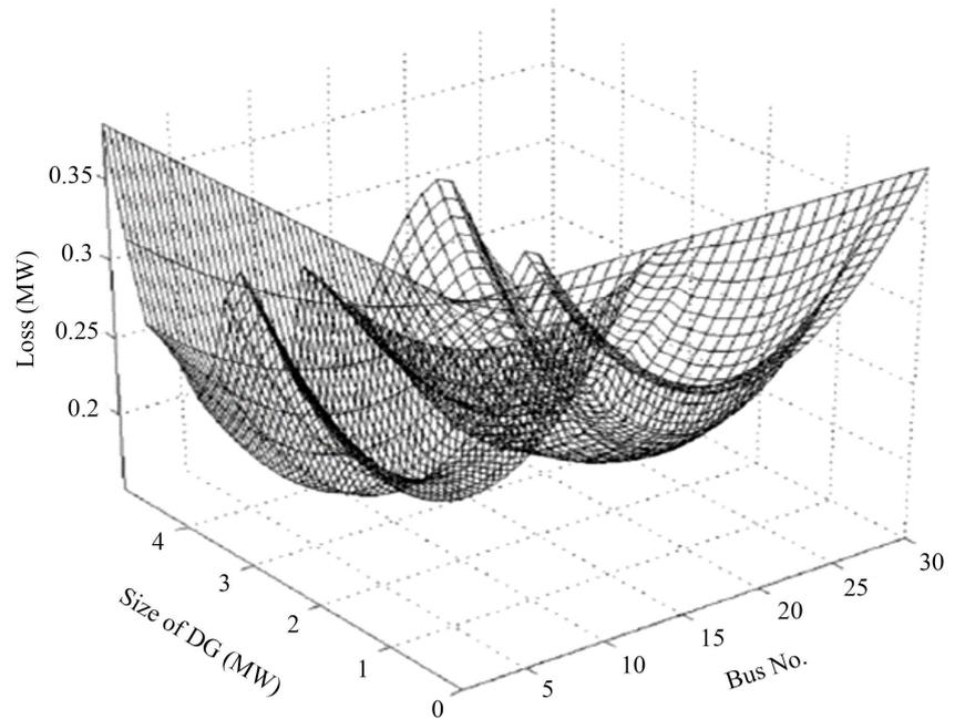
**Figure 2.** Effect of size and location of DG on system loss.
