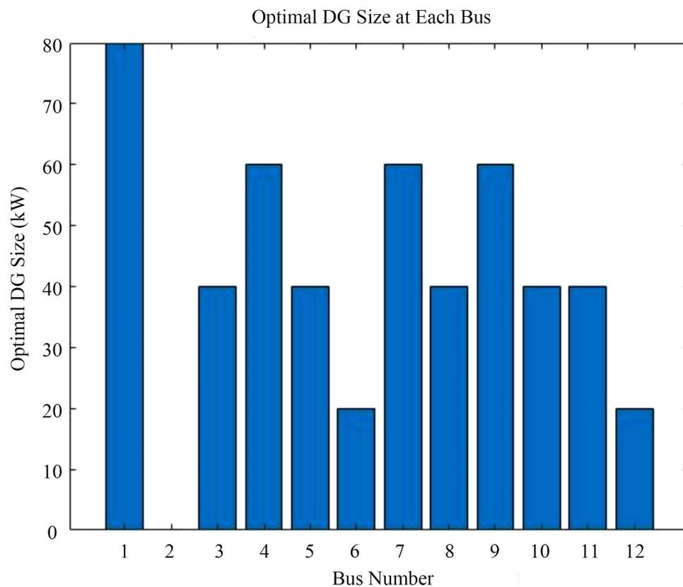
**Figure 8.** Optimal DG Sizes at estimated Buses based Sensitivity Optimization.
