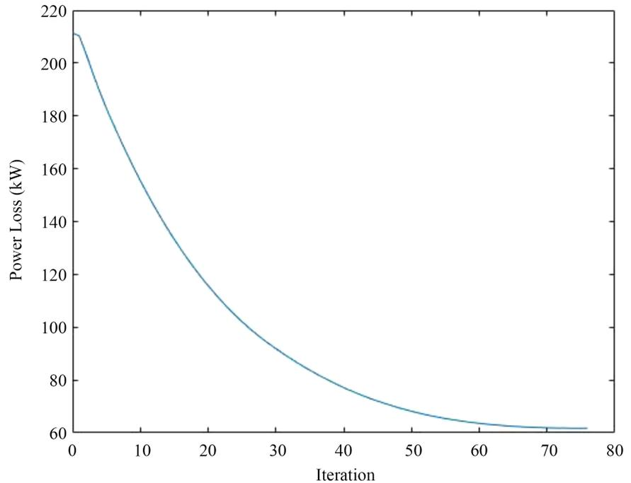
**Figure 7.** Power loss reduction for iterations in sensitivity-based DG placement.
