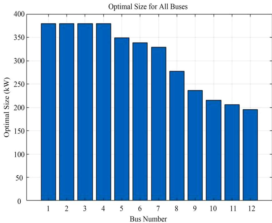
**Figure 5.** Optimum size of DG at all buses for 12 bus distribution system.
