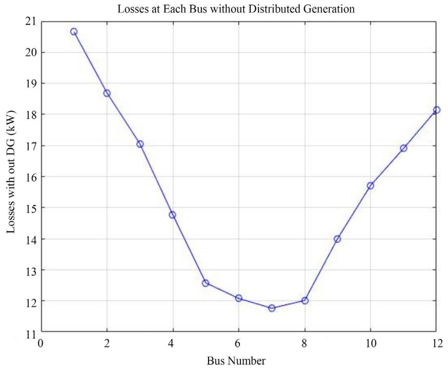
**Figure 4.** Losses of 12 bus distribution test system.
