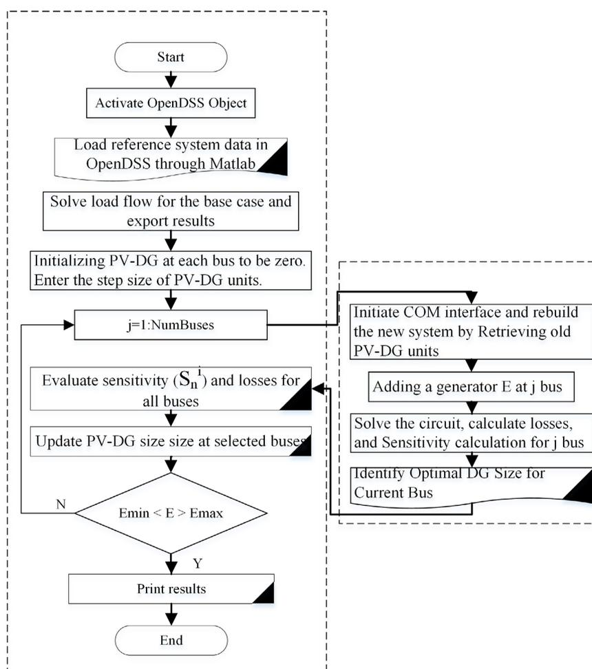
**Figure 3.** Chart of numerical method for PV-DG in distribution system.
