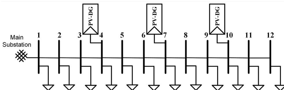
**Figure 11.** Single line diagram of 12-bus radial network.
