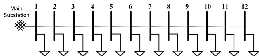
**Figure 1.** Single line diagram of the 12-bus radial distribution network.
