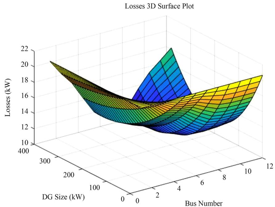
**Figure 6.** Losses, DG size of 12 bus distribution test system.
