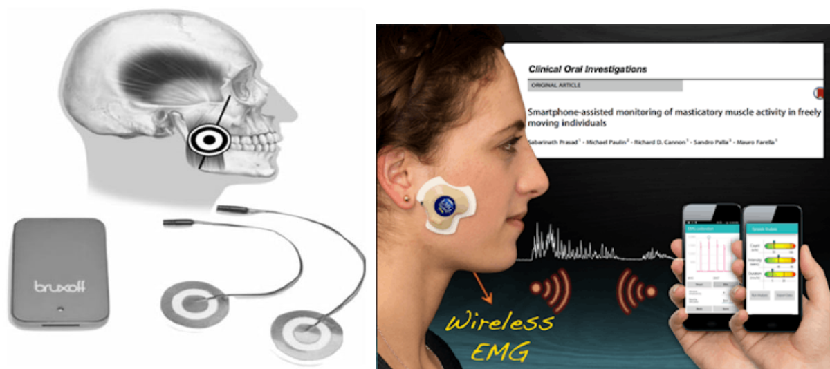
Figure 2. wireless electromyographic (EMG) device that patients wear on their jaws. The system was created by an international team of researchers, who detailed their development process and pilot study findings in Clinical Oral Investigations (January 4, 2019) [14].
