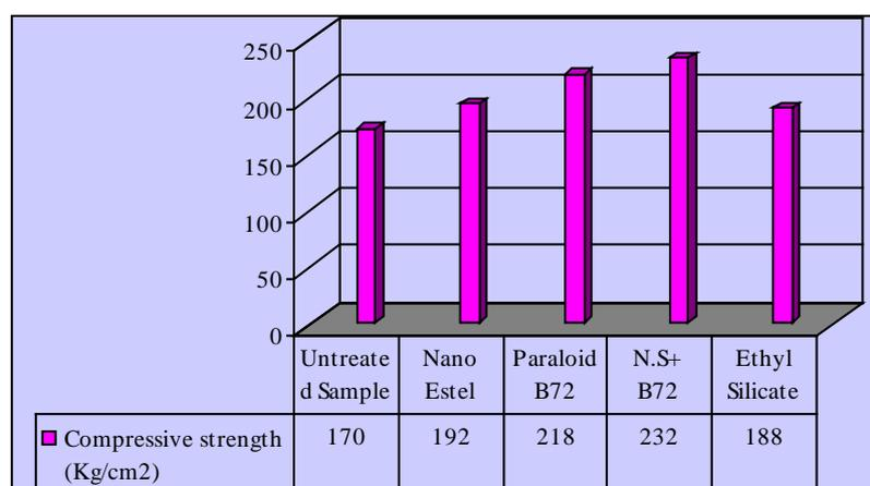
**Figure 11.** The mean values compressive strength of the treated samples.
