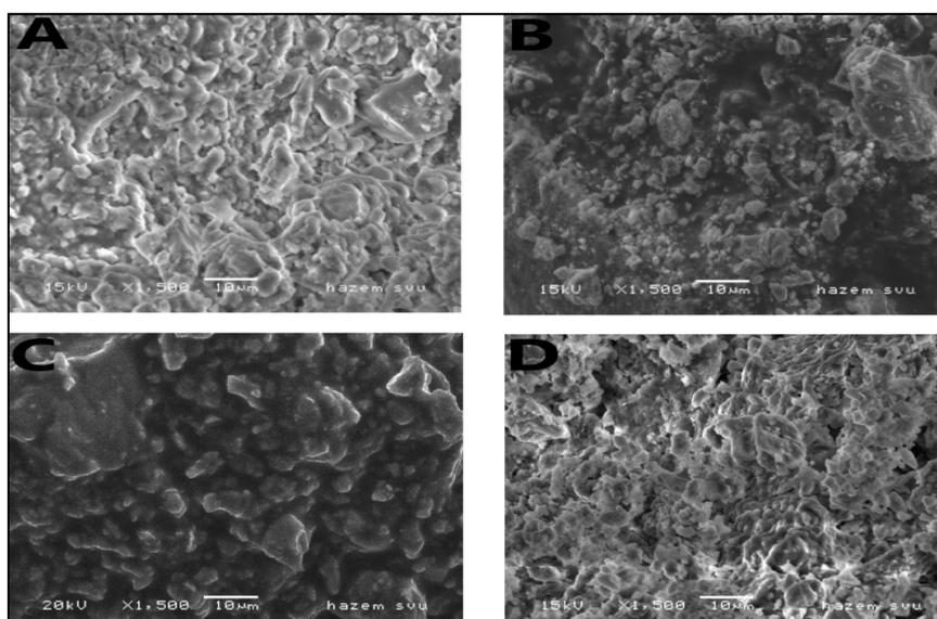
**Figure 8.** SEM micrographs of the treated sandstone samples. (A) The SEM examination of the treated samples with Nano Estel (1.500X). (B) The examination of the treated samples with Paraloid B-72 (1.500X). (C) The SEM examination of the treated samples with Nano Estel+B-72 (1.500X). (D) The examination of the treated samples with Ethyl Silicate (1.500X).
