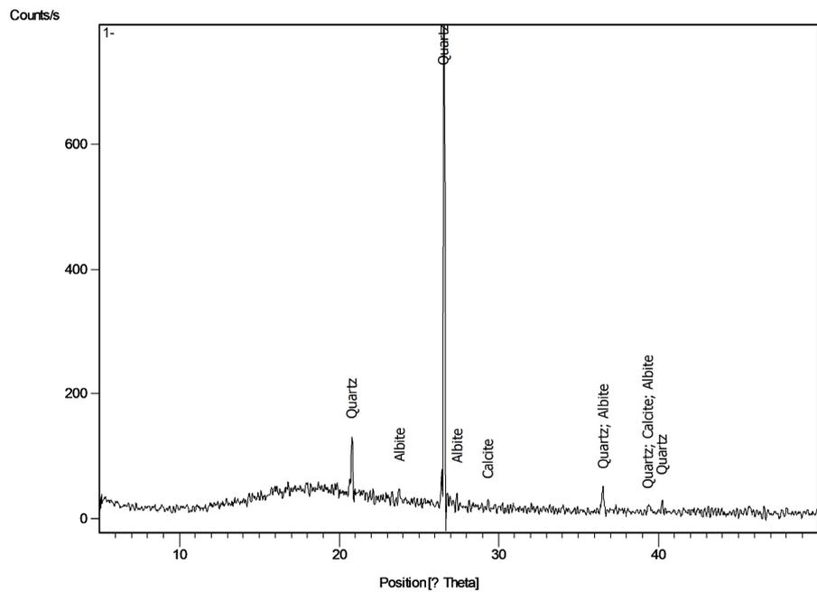
**Figure 7.** XRD pattern of the deteriorated sandstone.
