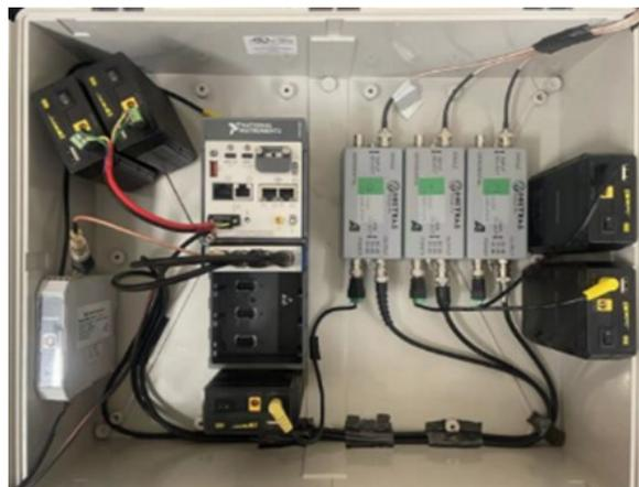
**Figure 1.** AE detection prototype.
