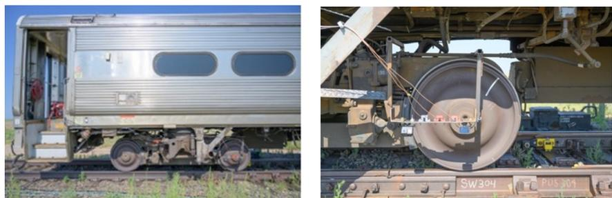
**Figure 10.** Testing car and sensor installation on RTT Loop.
