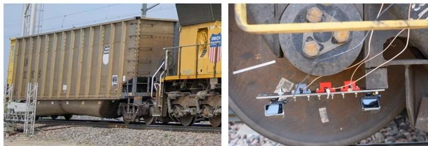
Figure 9. Testing vehicle and prototype installation on HTL loop.
