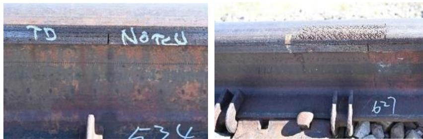
**Figure 6.** Defects in RDTF loop.
