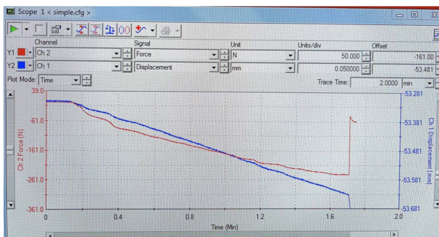
Figure 3. Real time data acquisition of displacement and force of the sample. Y axis is “displacement” and “force”. Redline represents force and blue line represents displacement. X axis is “time”. Values are negative as the position moves in a downward direction.
