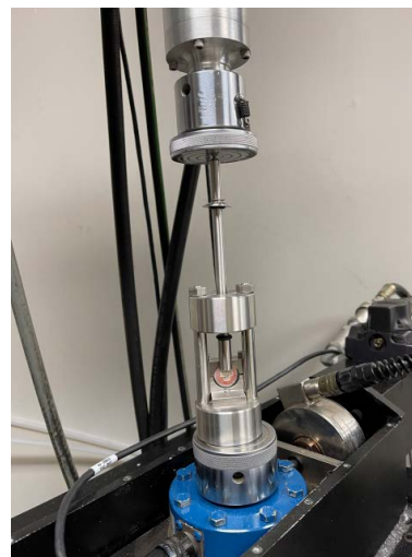
Figure 2. Testing jig mounted under the piston of the MTS universal testing machine.
