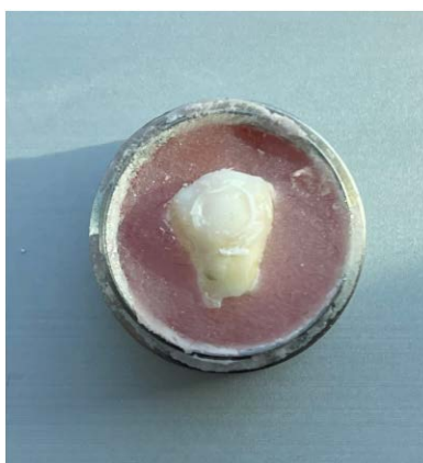
Figure 4. Sample after de-bond with remaining adhesive on enamel.
