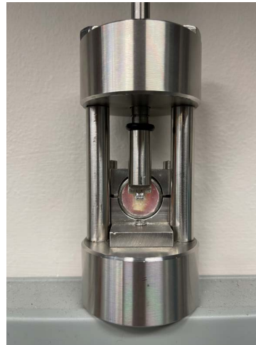
Figure 1. Mounting ring positioned in the custom Bencor Multi T testing jig.
