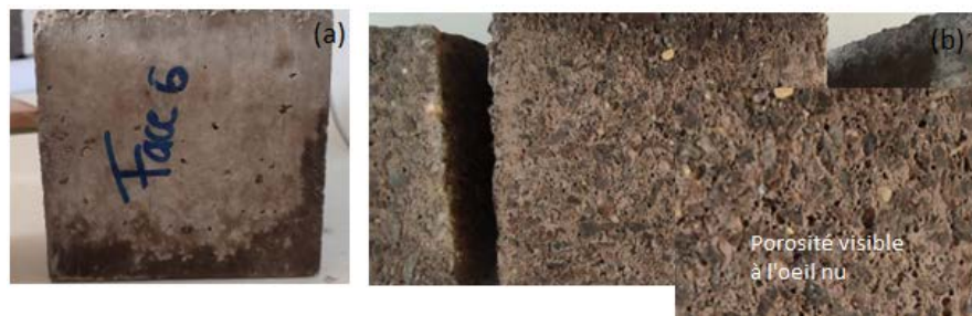
Figure 11. Cubic specimens 15 \times 15 \times 15 \text{ cm}^3 of concrete based on 50% slag. (a) After 7 days of curing in water (b) Cubic specimens 15 \times 15 \times 15 \text{ cm}^3 after 7 days immersion in 5% by mass of HCl.
