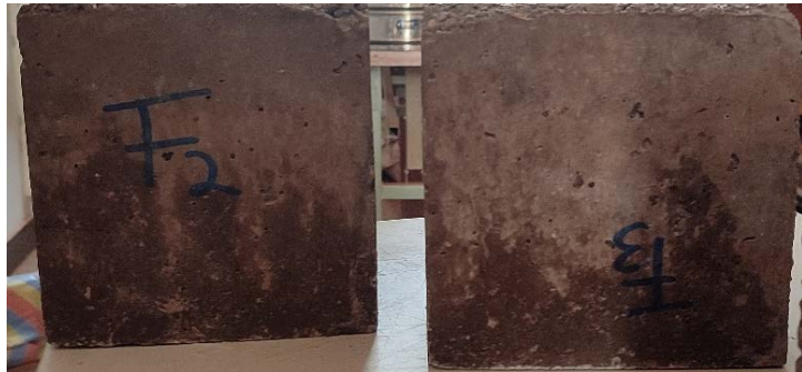
Figure 12. Cubic test tubes 15 \times 15 \times 15 \text{ cm}^3 of concrete based on 50% slag. Immersion of 7 days in 1% by mass of \text{Na}_2\text{SO}_4 .
