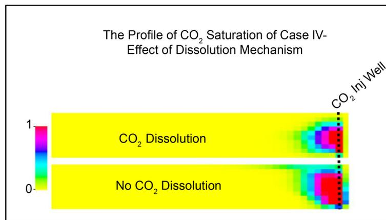
**Figure 8.** Effect of CO<sub>2</sub> dissolution mechanism on its saturation profile.
