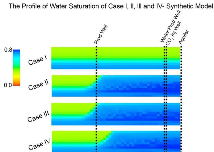
**Figure 4.** Comparison of water saturation profile for Case II, III and IV.
