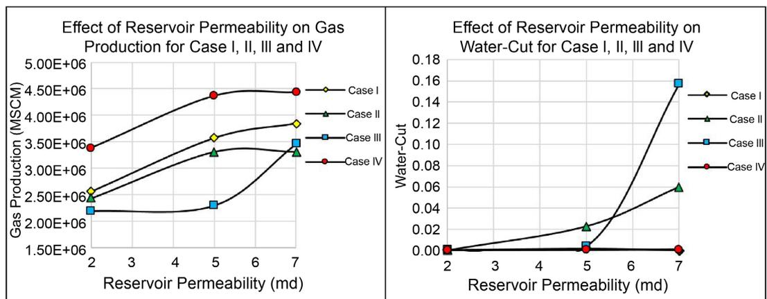
**Figure 2.** Comparison of cumulative gas production and water cut of Case I, II, III and IV for  $K_{xy} = 2, 5$  and  $7$  md (S.D = 0.3).
