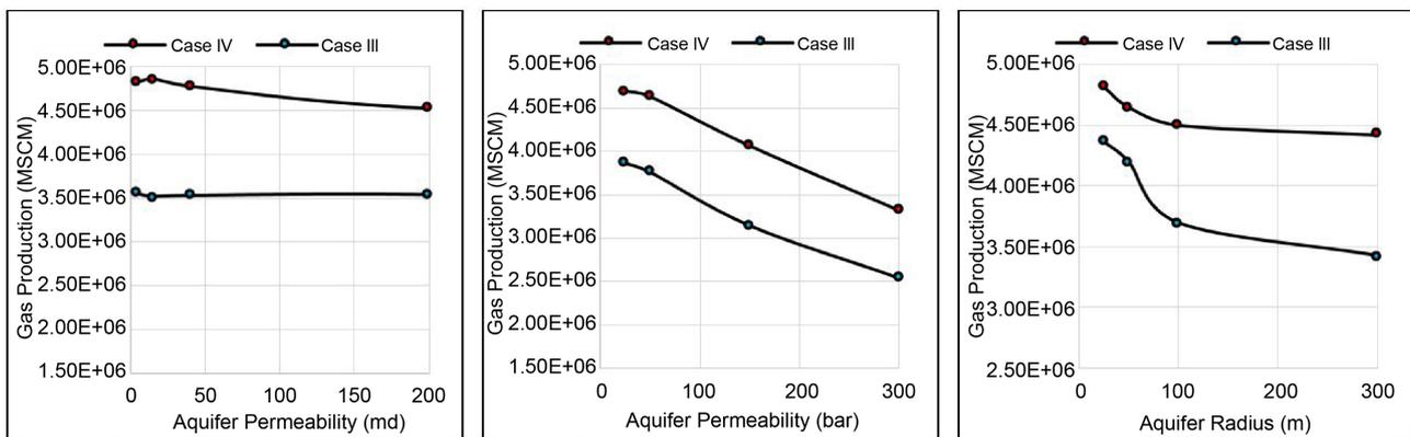
**Figure 6.** Effect of aquifer properties on gas production for Case III and IV and CO<sub>2</sub> production for Case IV.
