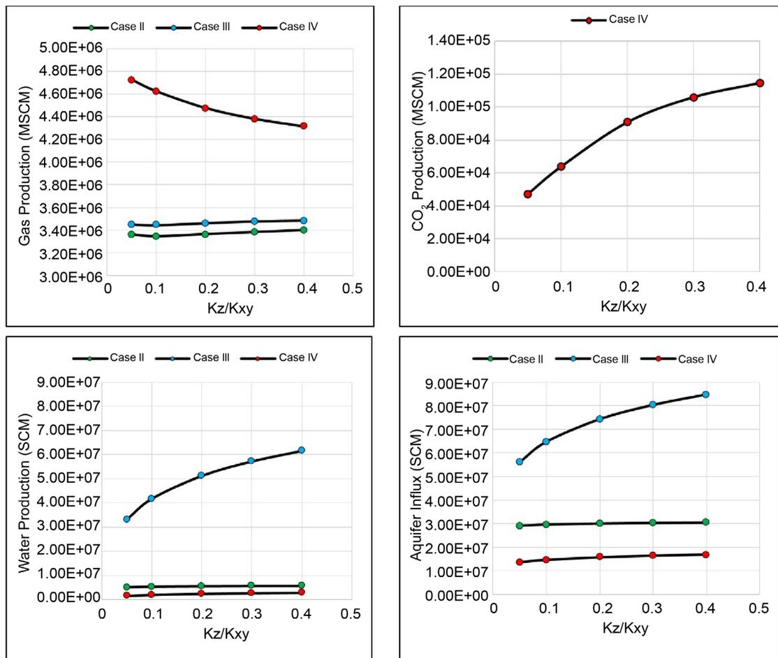
**Figure 5.** Effect of vertical to horizontal permeability on gas production, CO<sub>2</sub> production, water production and aquifer influx.
