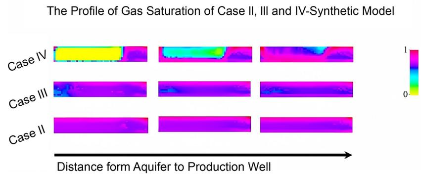
**Figure 3.** Comparison of gas saturation profile versus distance from aquifer for Case II, III and IV-cross section view.
