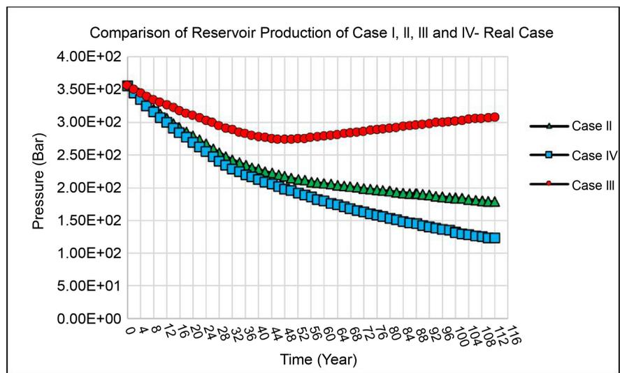
**Figure 11.** Comparison of reservoir pressure of Case I, II, III and IV-real case.
