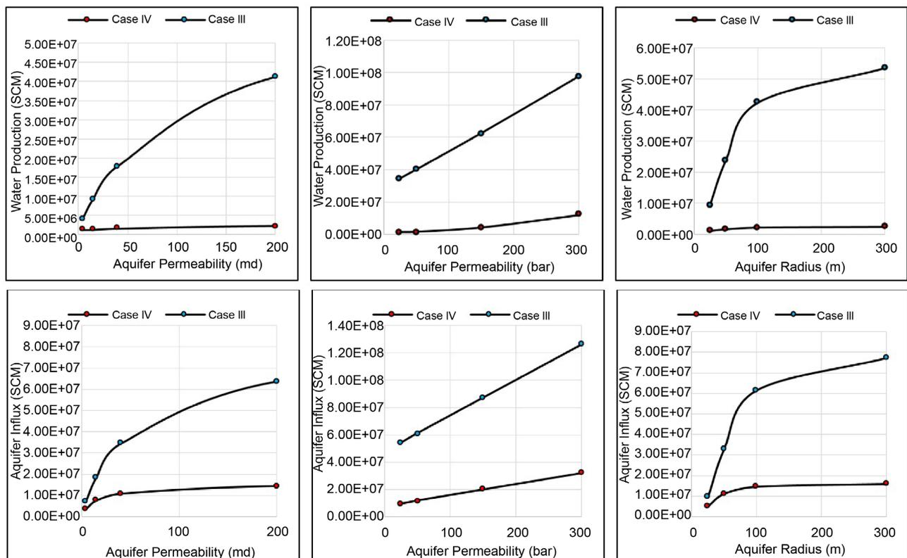
**Figure 7.** Effect of aquifer properties on water production and aquifer influx for Case III and IV.
