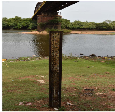
Figure 5. Showing the limnimetric scale for measuring the water level in the river bed.
