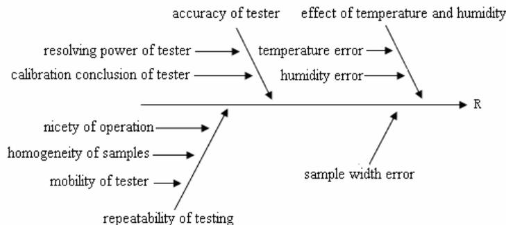
Fig. 1 The uncertainty sources of corrugating medium machine direction tensile strength
