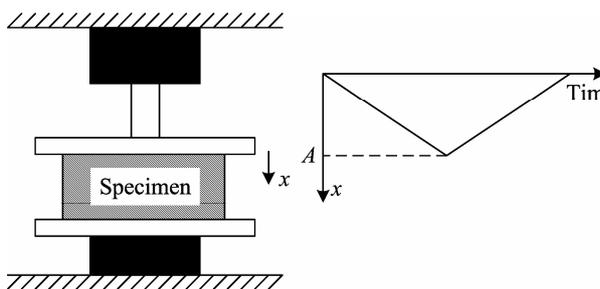
Figure 2. Schematic of the experiment set-up and imposed deformation
