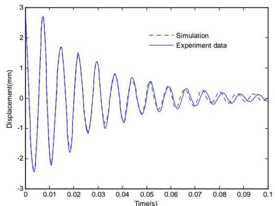
Fig. 5 Free response of the viscoelastic system
