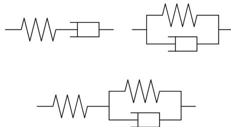
Fig. 4 Elementary models for viscoelasticity
