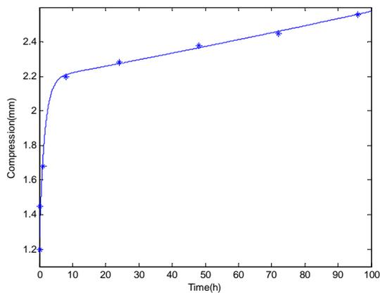
Fig. 1 Typical static creep under constant loading
