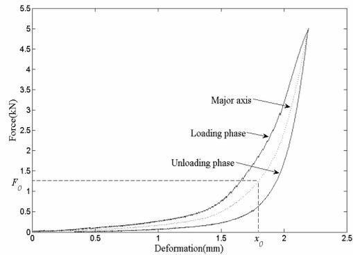
Fig. 3 The Force-Deformation curve of the quasi-static experiment
