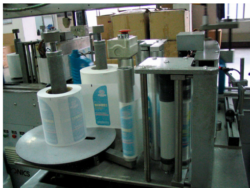
Figure 3. Packing mark is being printed by thermal transfer printing machine on the plastic drum with the paper being heated from its back.
