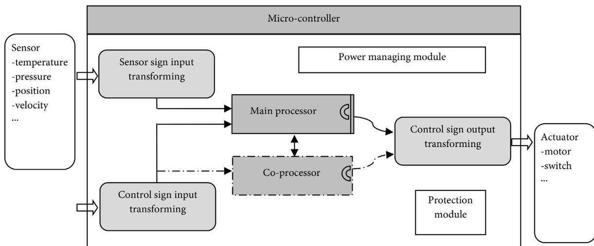
**Figure 1.** The general frame of embedded system.
