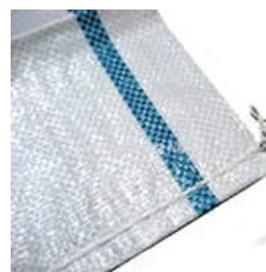
Figure 1. Common PP polywoven bag , lackluster surface
