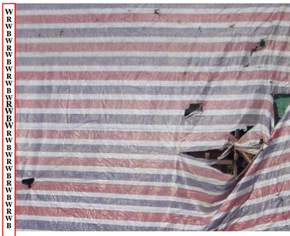
**Figure 2. Breakage holes on the aging tri-colored woven for enclosure**
