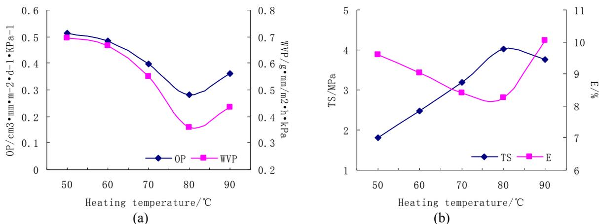
Figure4. Effect of heating temperature on main packaging properties of WPC film
