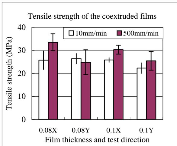
**Figure 5. Tensile strength of two coextruded films with 0.08mm and 0.10mm thick at two different test speeds in perpendicular directions.**
