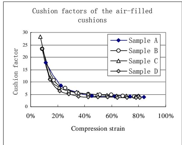
**Figure 3. Cushion factors vs. strain of four types of cushion samples**
