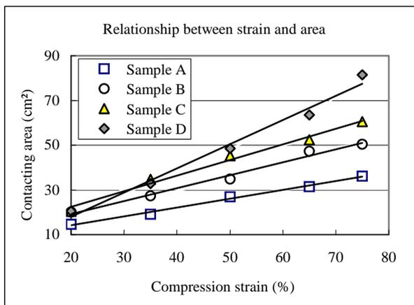
**Figure 2. Linear relationship between contacting area of the cushion samples and compression strains.**
