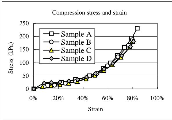
**Figure 1. Compression stress and strain of four types of cushion samples.**
