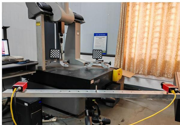
**Figure 7.** Target position and attitude Measurements using CMM and MCS.
