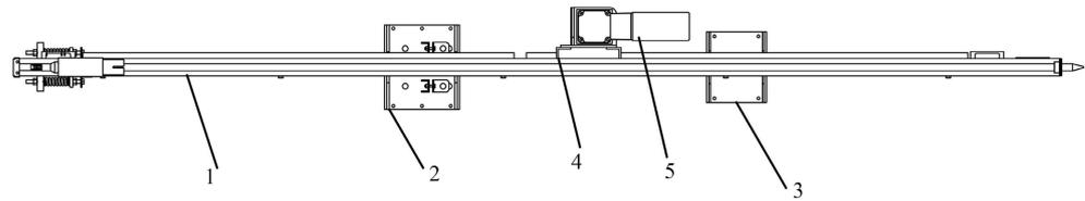
**Figure 3.** Structural diagram of the auxiliary carriage mechanism. 1. Main Beam, 2. Fixed bracket on main beam, 3. Fixed bracket under main beam, 4. Walking Motor Mounting Plate, 5. Walking Motor.
