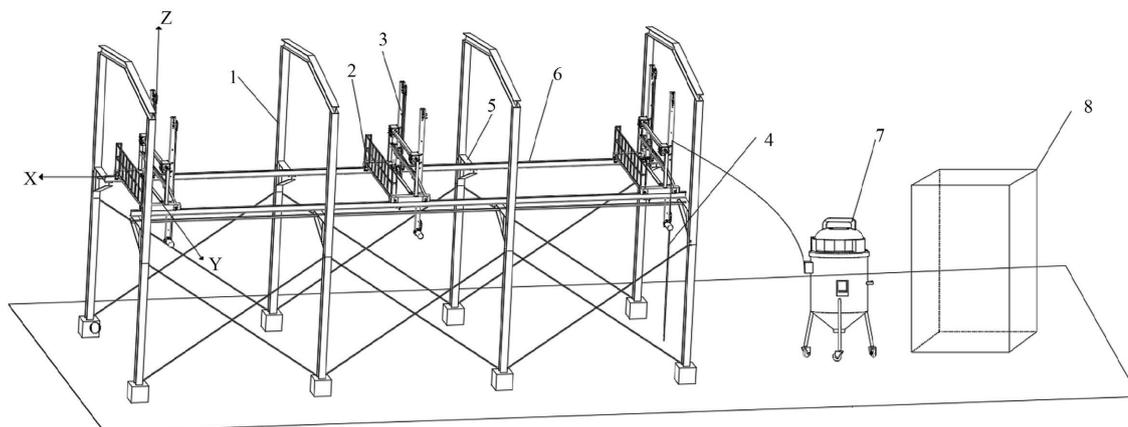
**Figure 1.** Structural diagram of the multi-rod sampling machine. 1. Pillars, 2. Main Carriage Mechanisms for Sampling, 3. Auxiliary Carriage Mechanisms for Sampling, 4. Sampling Rods, 5. Reinforcements, 6. Cantilever Beams, 7. Grain Suction Devices, 8. Control Cabinet.
