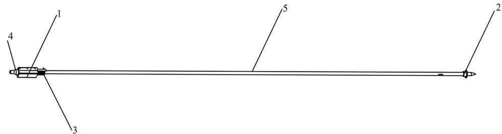
**Figure 4.** Structural diagram of the sampling rod. 1. Connecting Plate, 2. Roller Bearing, 3. Spring, 4. Sleeve, 5. Sampling Rod.
