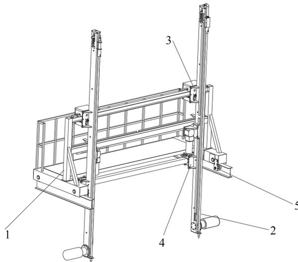
**Figure 2.** Structural diagram of the main carriage mechanism. 1. Main Carriage Frame, 2. Sampling Machine Vertical Arm, 3. Sampling Carriage Lateral, 4. Movement Upper Guide, 5. Sampling Carriage Lateral Movement Lower Guide, 6. Anti-, 7. Derailment Device.
