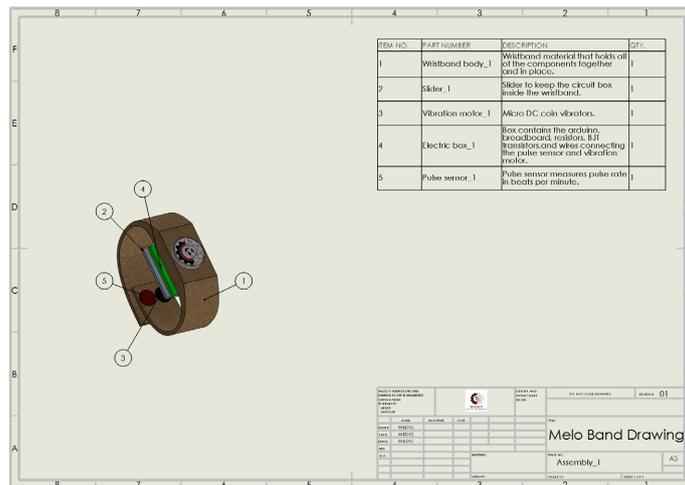
**Figure 3.** Bill of Materials for the Device.
