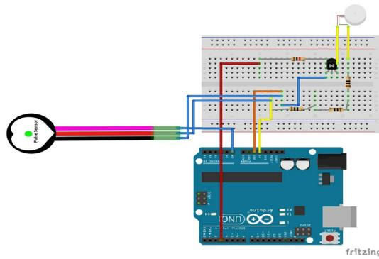
**Figure 2.** Electronic design of the wristband prototype.
