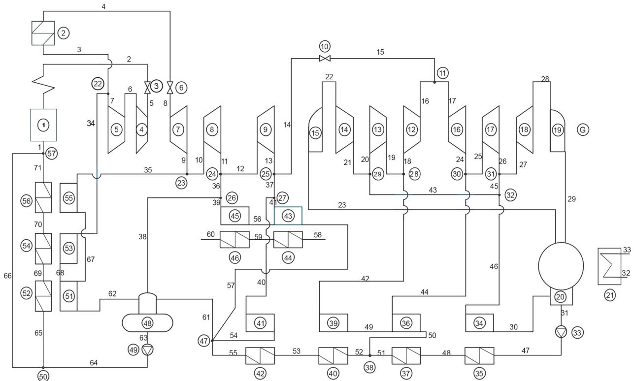
**Figure 3.** Structural process scheme for the reference steam block.
