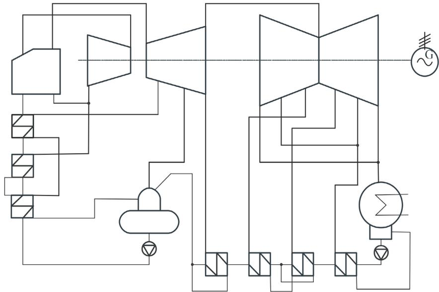
**Figure 2.** Standard marked process scheme of a steam block for the production of electricity.
