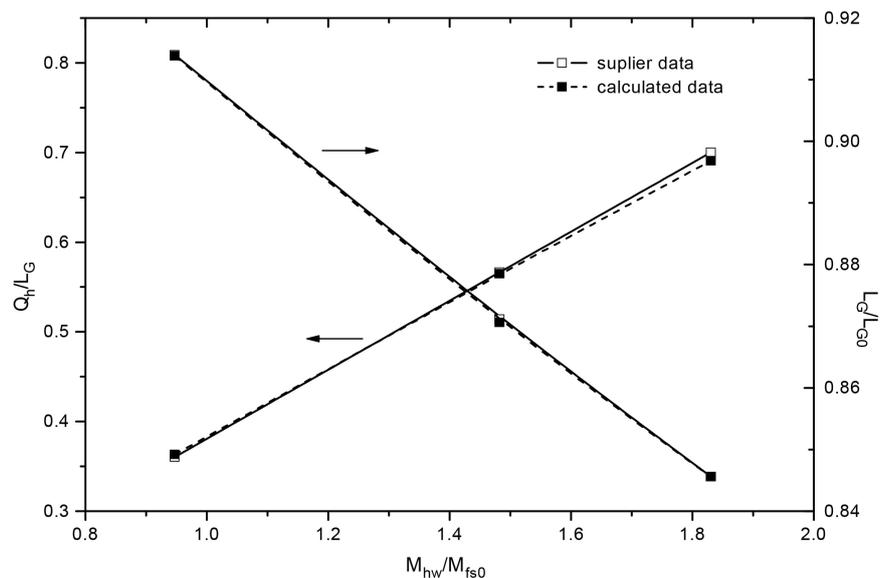
**Figure 9.** Comparison of calculation results and supplier’s data for the given regimes of combined production of heat and electricity.
