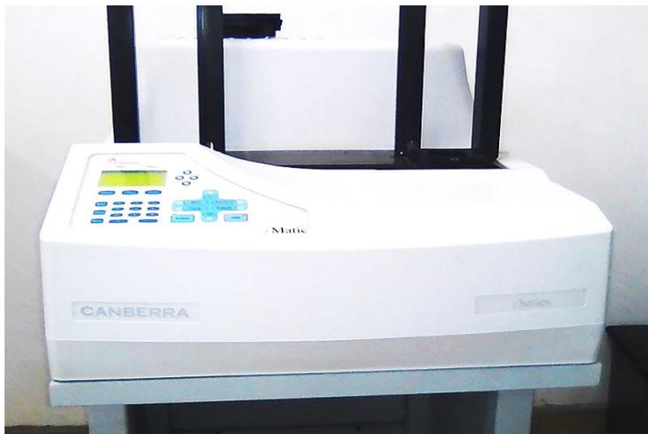
**Figure 2.** Picture of the automatic Alpha/Beta counting system (Canberra iMatic™).
