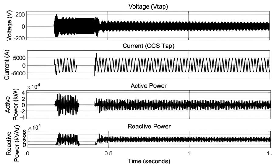
**Figure 14.** CCS tap node with fault.
