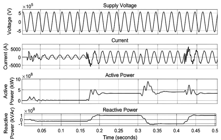
**Figure 13.** Supply parameters under CCS node fault.
