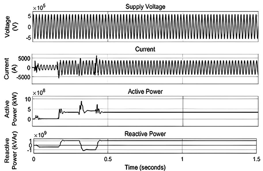
**Figure 6.** Supply parameters.
