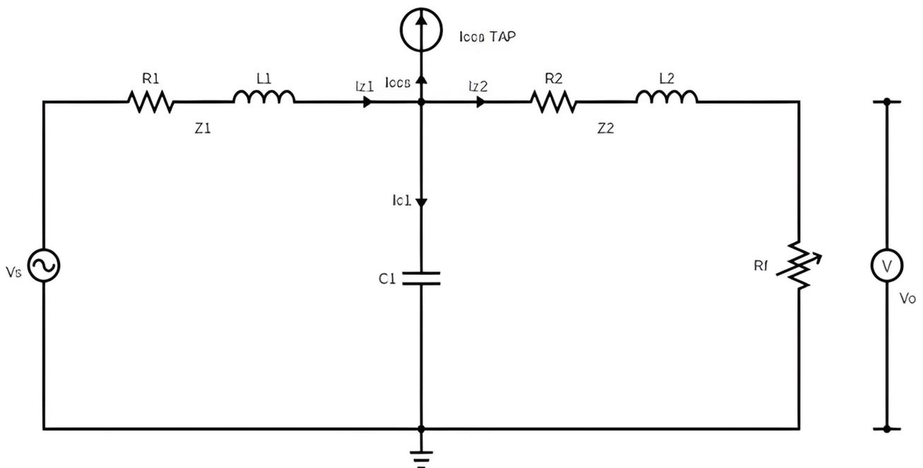
**Figure 4.** Transmission line CCS system equivalent circuit with power tapping.
