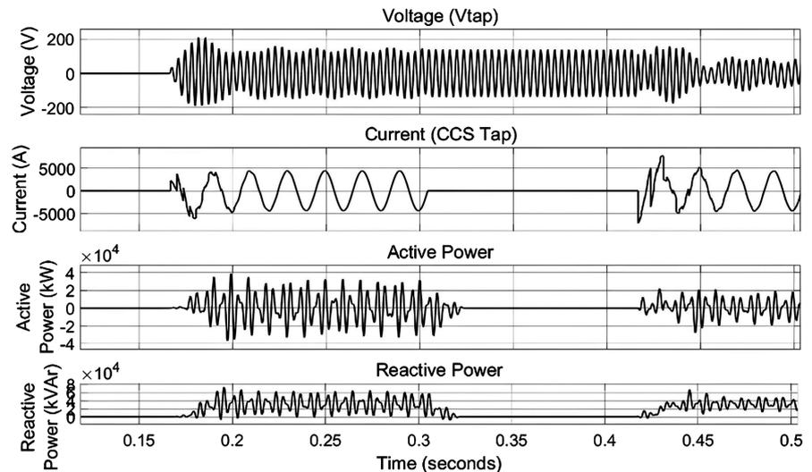
**Figure 15.** CCS tap with fault—expanded span.
