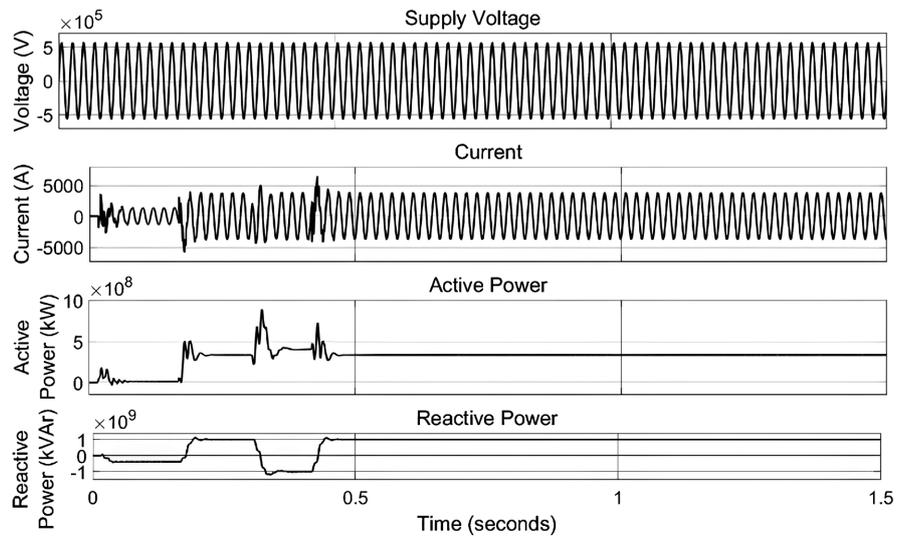
Figure 12. Supply parameters under fault conditions.
