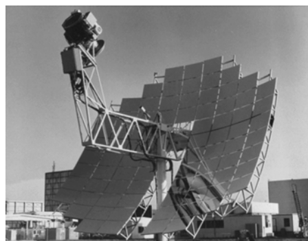
Figure 5. 25 kW dish stirling engine driven by solar power generation system
