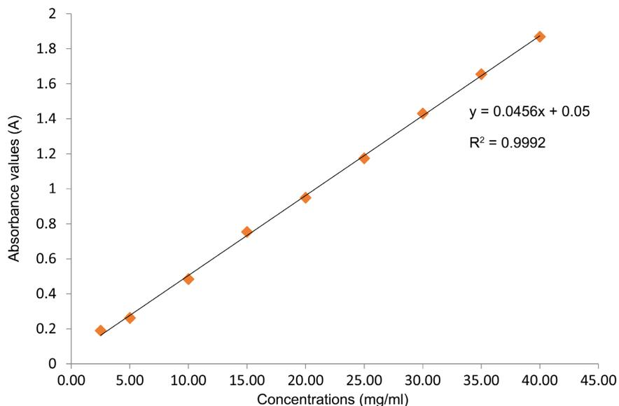
**Figure 4.** Calibration curve of 2-acetoxy benzene carboxylic acid in methanol.
