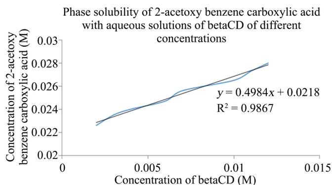
**Figure 5.** Phase solubility diagram of 2-acetoxy benzene carboxylic acid with aqueous solutions of  $\beta$ -CD of different concentrations.
