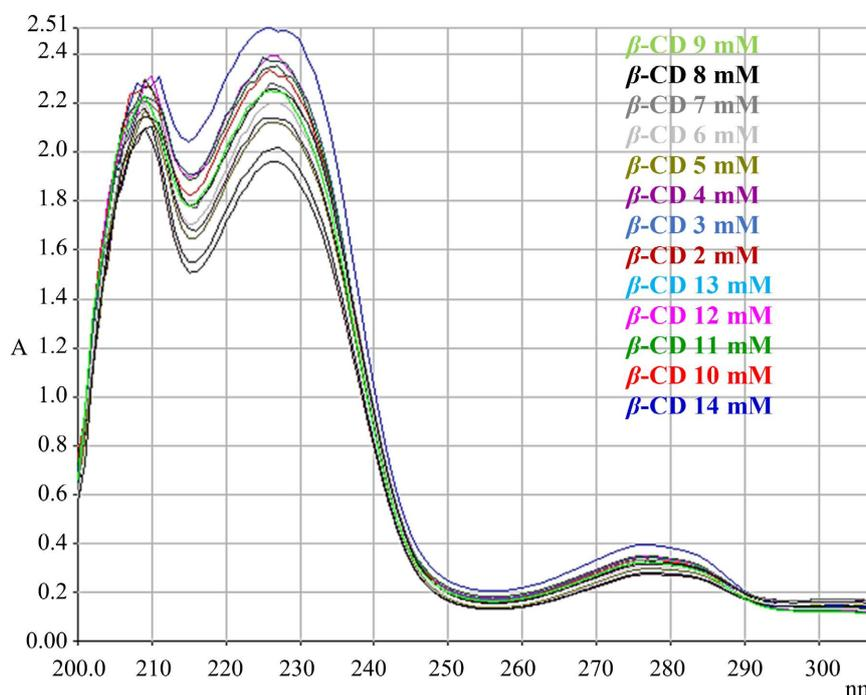
**Figure 7.** UV spectra of 2-acetoxy benzene carboxylic acid in aqueous  $\beta$ -cyclodextrin solutions of different concentrations (1 - 14 mM).
