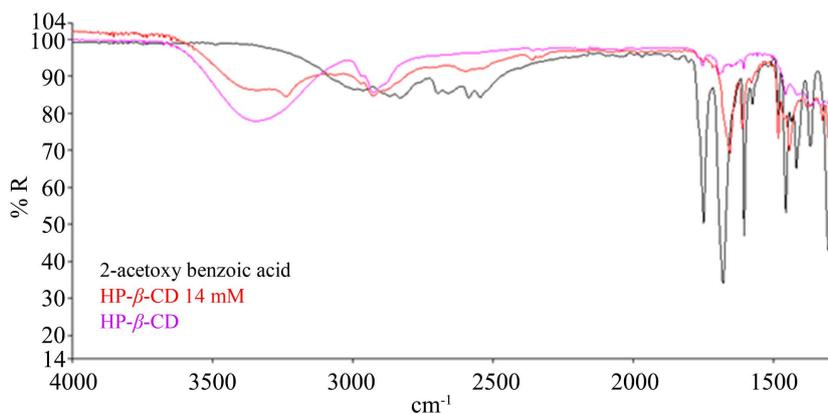
**Figure 11.** FTIR spectra of 2-acetoxy benzene carboxylic acid and 2-acetoxy benzene carboxylic acid complex with 2-hydroxypropyl- $\beta$ -cyclodextrin (14 mM).
