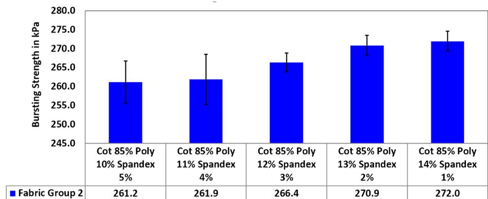
**Figure 5.** A graphical display of the bursting strength of Group 2 Fabrics.
