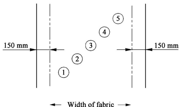
**Figure 2.** The position of the sample collection from fabric.
