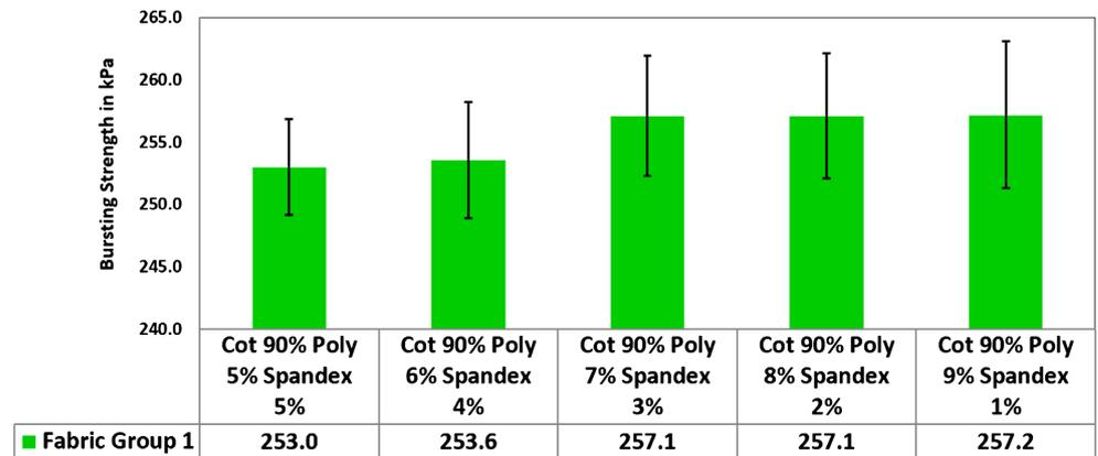
**Figure 4.** A graphical display of the bursting strength of Group 1 Fabrics.
