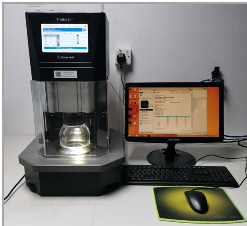
**Figure 1.** The digital bursting strength tester.
