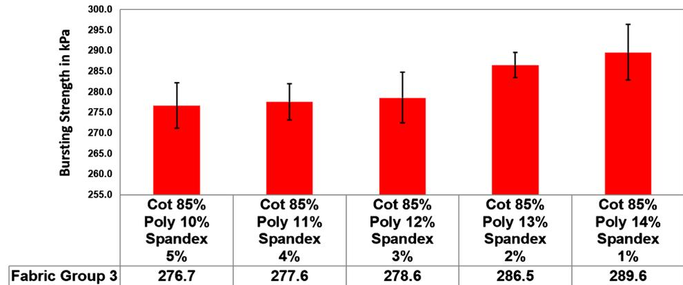
**Figure 6.** A graphical display of the bursting strength of Group 3 Fabrics.
