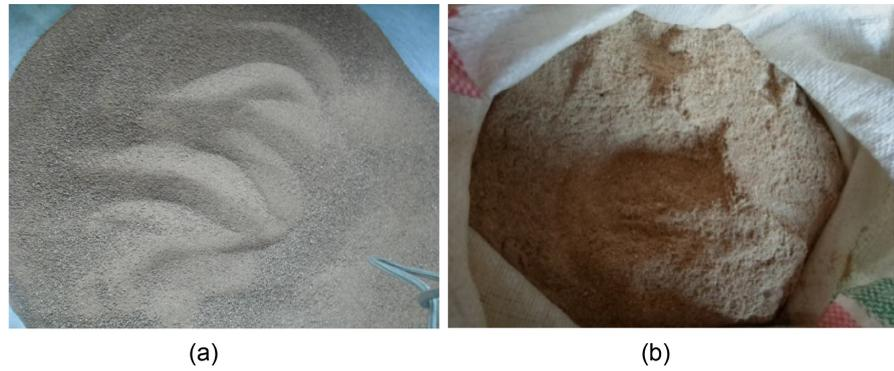
**Figure 2.** Materials used for analysis: (a) Clay sample from the site; (b) Rice husks.
