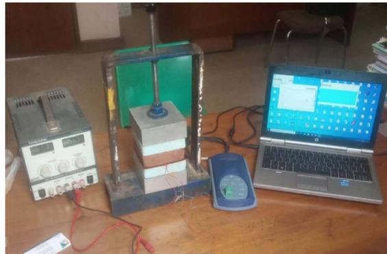
**Figure 5.** The testing instruments used for measuring the thermal properties.
