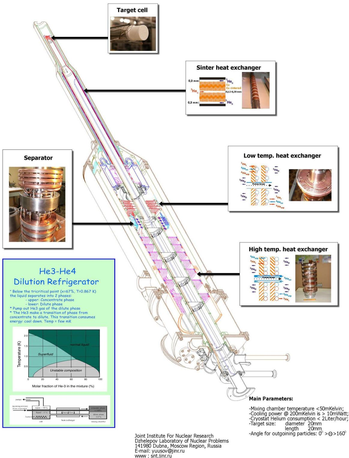
Figure 11. Main units and parameters of the polarized target cryostat in Mainz.
