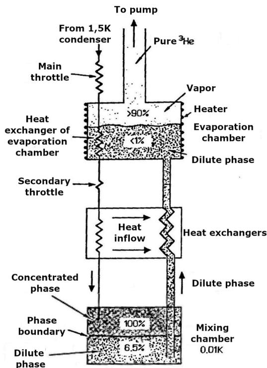
**Figure 1.** Typical diagram of the  $^3\text{He}/^4\text{He}$  refrigerator.
