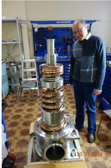
**Figure 12.** Cryostat for Bonn is almost completed. A. B. Lazarev.
