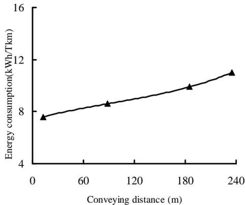
Figure.5 Trend of energy consumption in different conveying distance
