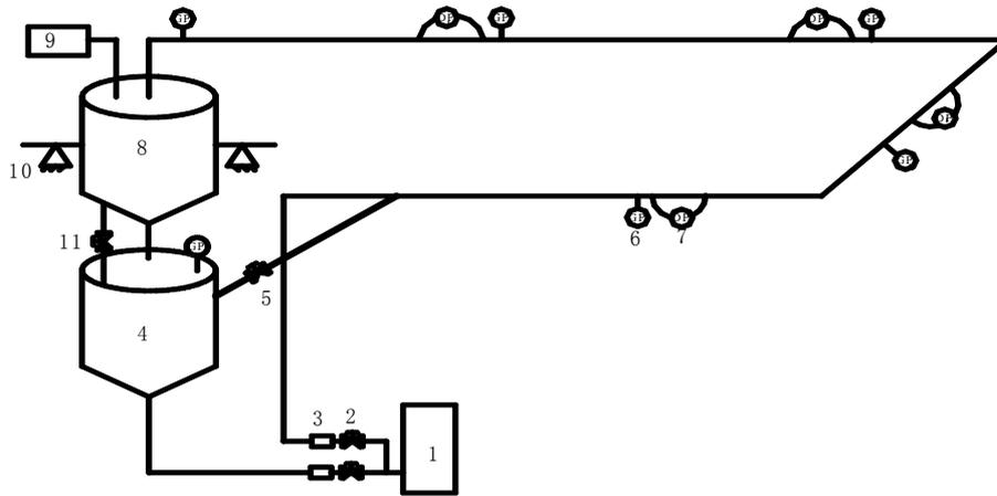
1. air supply 2. gas valve 3. gas flux apparatus 4. feeder vessel 5. solid injector valve 6,7. static/differential pressure cell 8 receiver vessel 9 dust collector 10. weight balance 11. balanced valve
