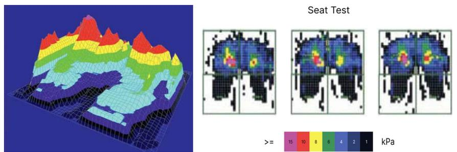
Figure 11. Car seat pressure distribution.
