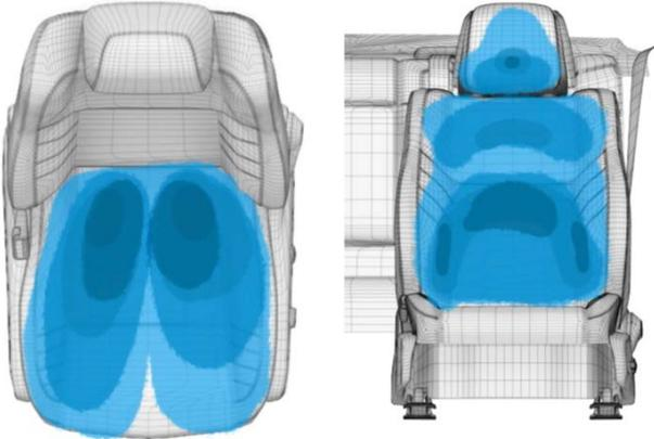
**Figure 12.** Car seat pressure distribution measurement.
