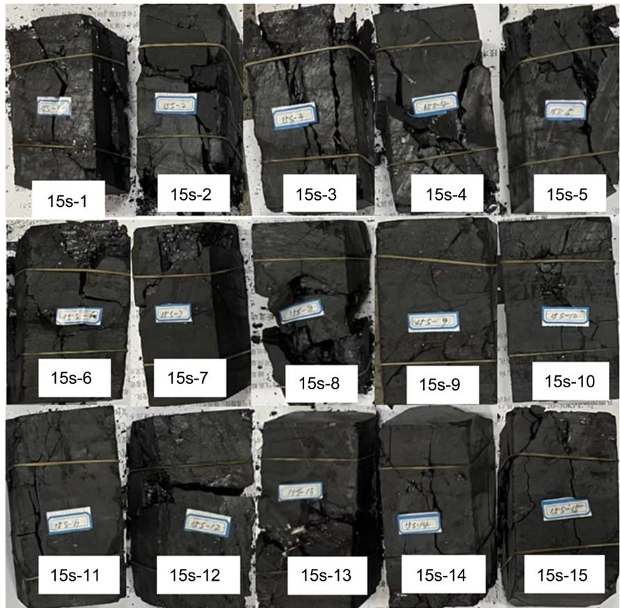
Figure 5. Failure mode of the fifteen coal samples.
