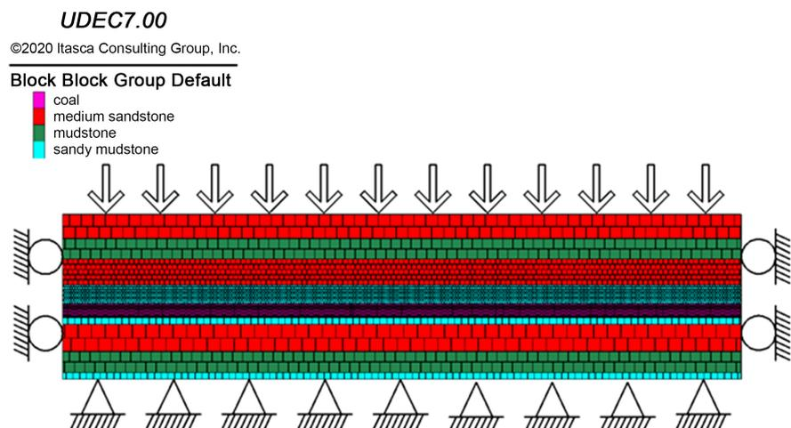
**Figure 3.** Comprehensive release of the working surface advanced support pressure UDEC numerical model.
