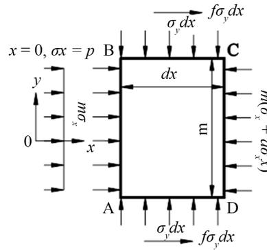
**Figure 2.** The force state of the microstructure in the limit equilibrium zone of the slope.
