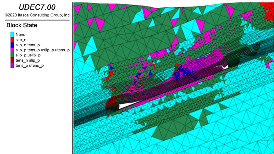
**Figure 8.** Cloud view of lateral plastic zone at header face.
