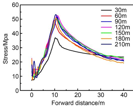
**Figure 4.** The pressure distribution of the advanced support of the working surface of the comprehensive discharge at different mining distances.
