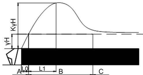
H—Depth of burial;  $\gamma$ —Bulk capacity; A—Decompression zone; L0—Sheet gang zone; L1—Plastic zone; B—Augmentation zone; C—Primary rock stress zone.
