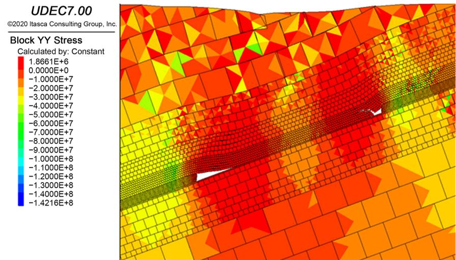
**Figure 7.** Lateral support pressure UDEC model Lateral support pressure cloud at the heaving face.
