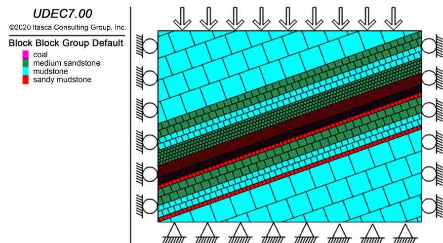
**Figure 6.** Comprehensive discharge work surface lateral support pressure UDEC model.
