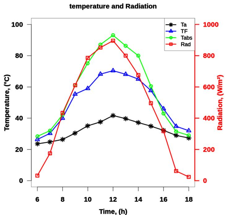
**Figure 3.** Curve of different temperatures at the sensor.
