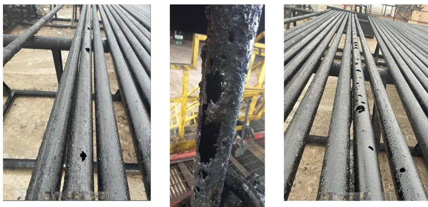
**Figure 3.** Visuals of corroded subsurface production tubing at end of life.
