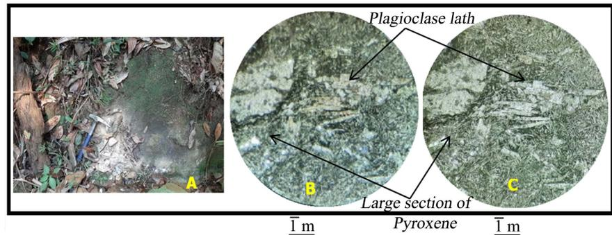
**Figure 4.** (A) Dolerite sample (Kinzoki region). (B) and (C) Thin section microscopic view (LN and LP) of dolerites showing plagioclase laths.
