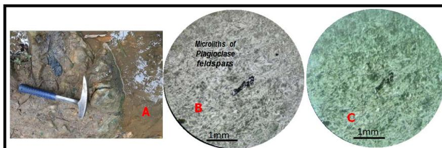
**Figure 3.** (A) Basalt outcrop; (B) and (C) Thin section microscopic view (LN and LP) of Basalt from the Kinzoki region.
