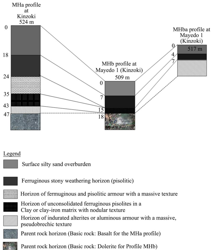
**Figure 5.** Presentation of the MHa, MHb and MHba weathering profiles and their schematic correlation *in situ* in the study area.
