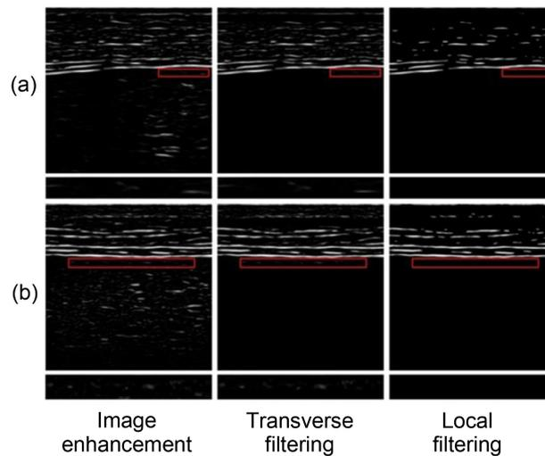
**Figure 5.** The effect of transverse filtering combined with local filtering.
