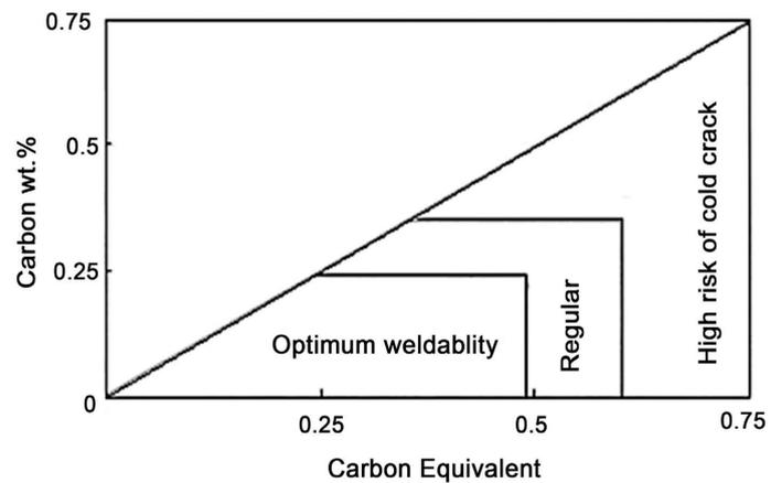
**Figure 1.** Carbon content/equivalent carbon diagram showing optimum, consistent weldability zone and high risk of cold cracking [16].
