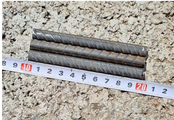
**Figure 2.** Bars 10 cm long for mass determination.
