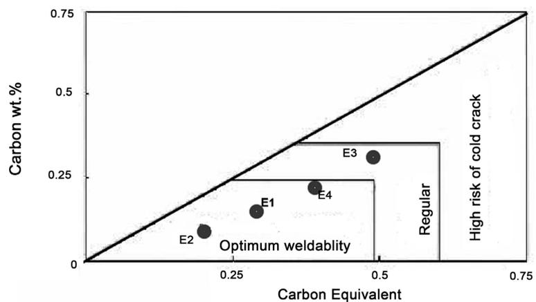
**Figure 3.** Placement of the samples studied (E1, E2, E3 and E4) in the diagram according to the values of C and Ceq.
