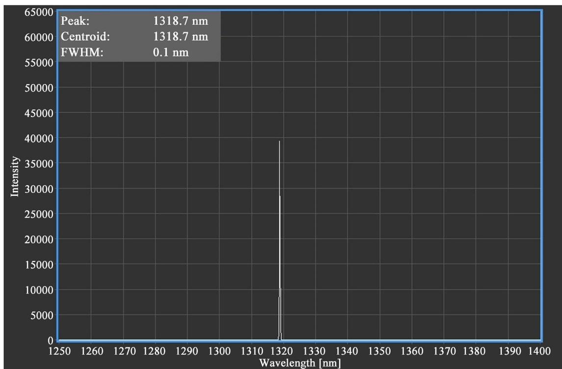
**Figure 4.** Laser spectrum when output power is 91.1 W.
