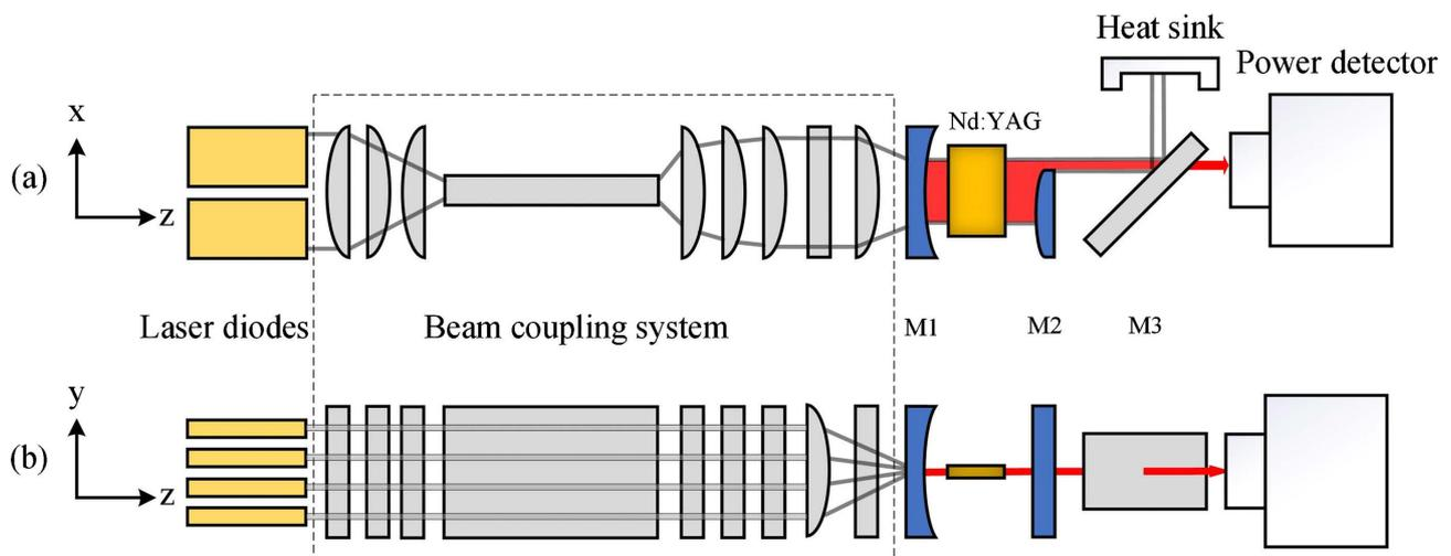
**Figure 1.** Schematic of experimental setup. (a) In the horizontal direction; (b) In the vertical direction.
