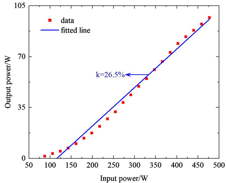
**Figure 2.** Laser output power versus pump power.
