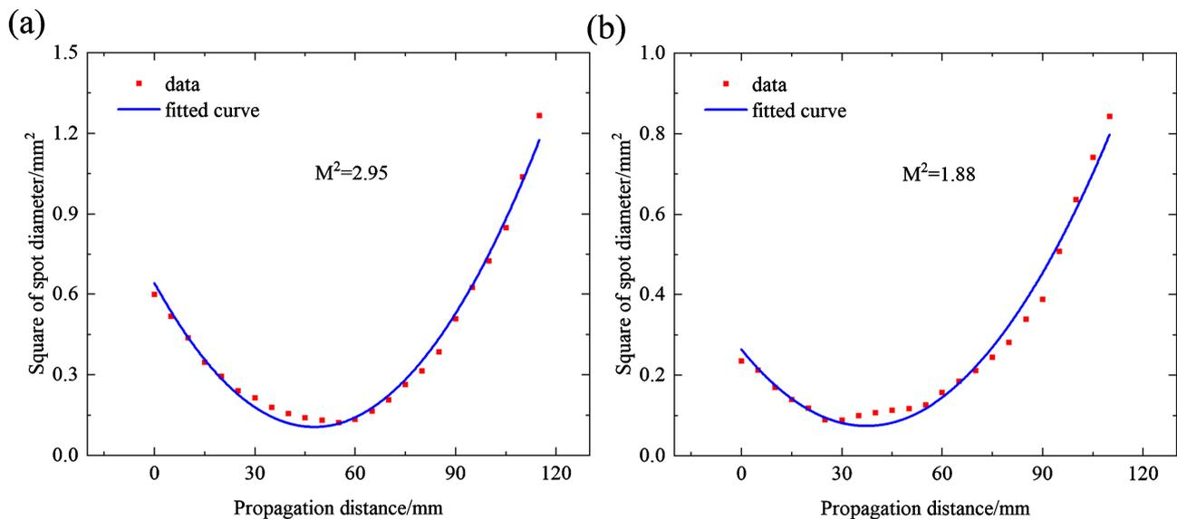
**Figure 3.** Laser beam quality factors. (a) In the stable direction; (b) In the unstable direction.
