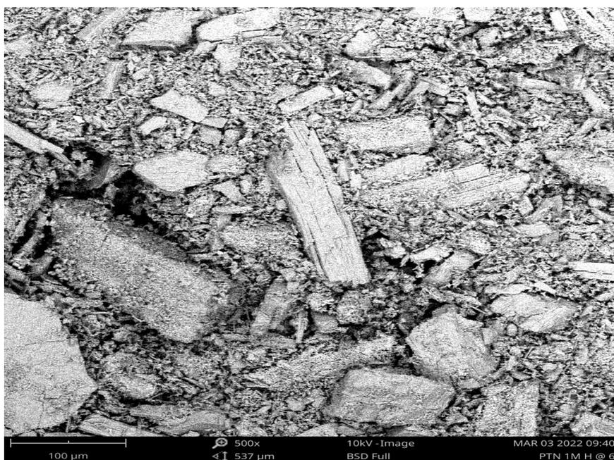
**Figure 6.** Scanning electron micrograph of Acid treated *Pila globosa* shell Calcined at 600°C The micrograph of raw (PTW1M).
