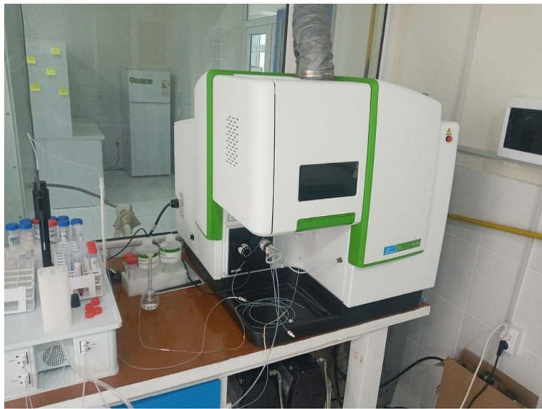
**Figure 3.** ICP-OES laboratory instrument. (ICP-OES is an optical emission spectrometer based on inductive plasma. The device for high-precision (0.001 mg/l) measurement of elements from solutions in argon flow.)
