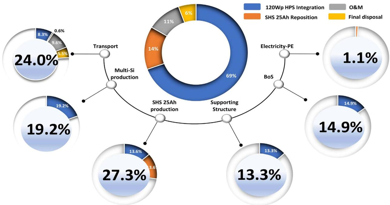
Figure 6. Carbon footprint distribution for each process involved for the production of 1 kWh of electricity using 120Wp HPS.
