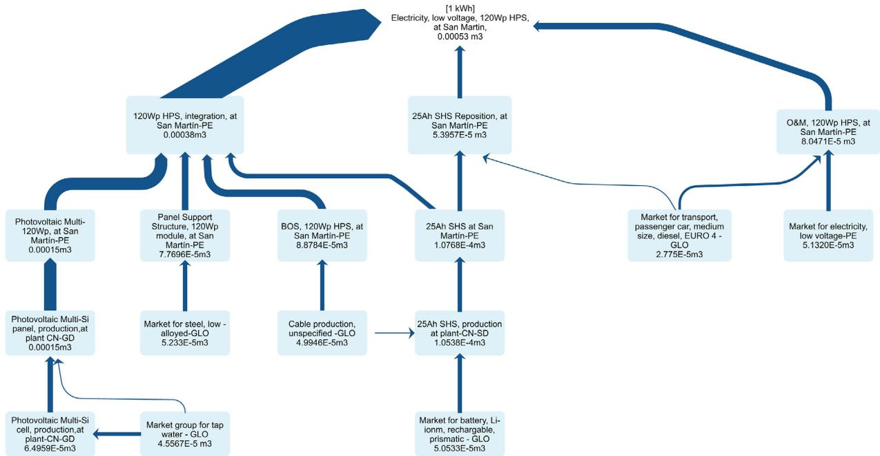
Figure 7. Sankey diagram of water footprint category for the production of 1 kWh of electricity using 120Wp HPS.
