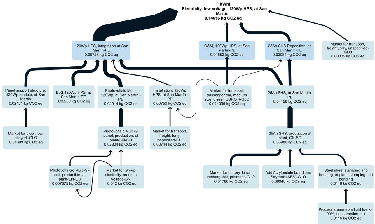
Figure 5. Sankey diagram for climate change category for the production of 1 kWh of electricity using 120Wp HPS.
