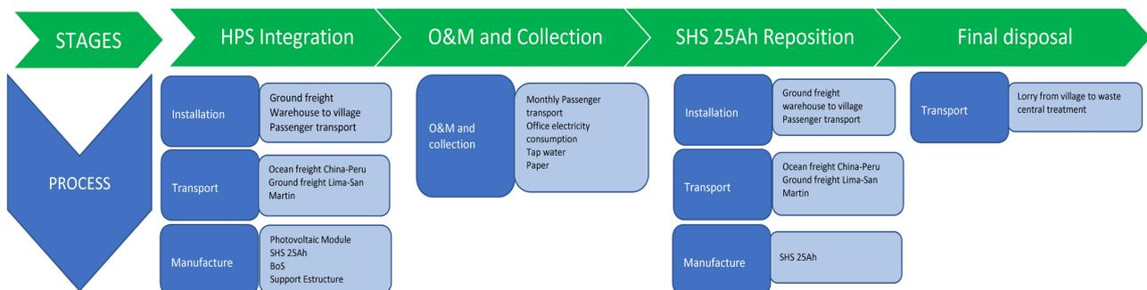
**Figure 3.** Stage and process for a 1 kWh HPS production.
