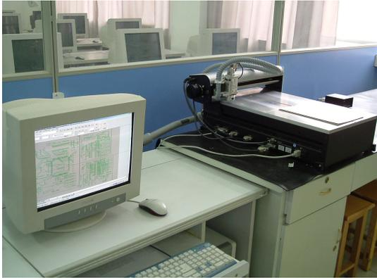
Figure 4.2 PCB graving equipment
