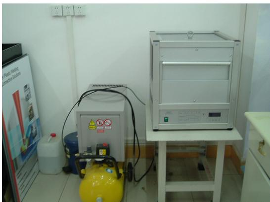
Figure 4.4 PCB laminating equipment
