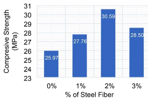
**Figure 3.** Effect of steel fiber on the average compressive strength of concrete at 28 days.
