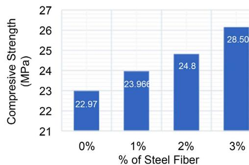
**Figure 2.** Effect of steel fiber on the average compressive strength of concrete at 7 days.
