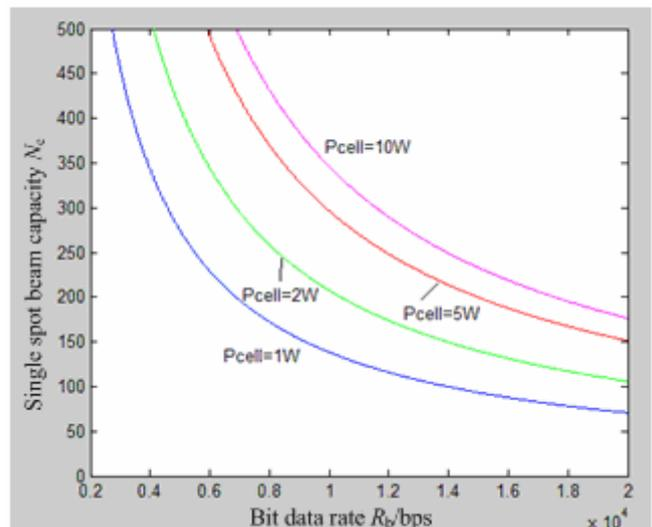
Fig. 3 Relation between system capacity and bit data rate in TD-CDMA scheme
