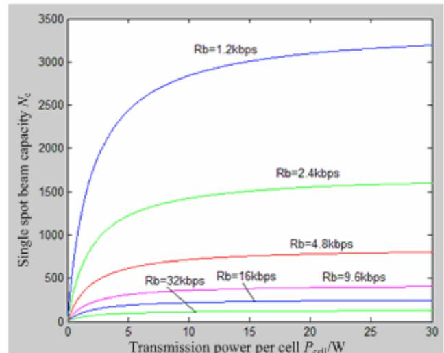
Fig. 2 Relation between system capacity and transmission power in TD-CDMA scheme.
