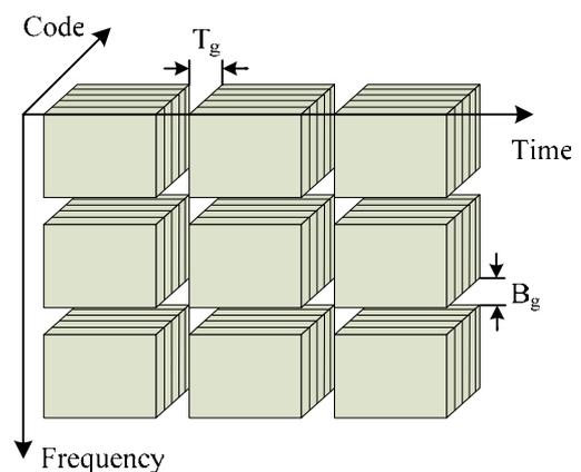
Fig. 1 Channel division of the TD-CDMA scheme.
